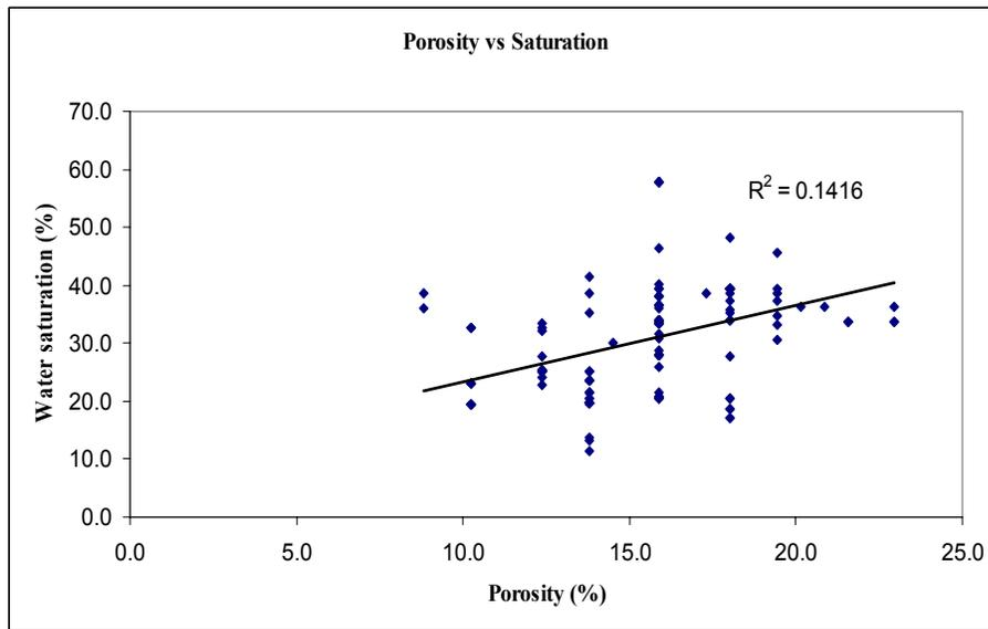
Figure B.8 - Porosity vs. Saturation Graph for Field B
