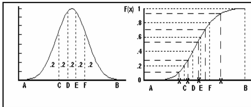
Figure 2.3- Sampling Results by LHC and Random Sampling Methods
