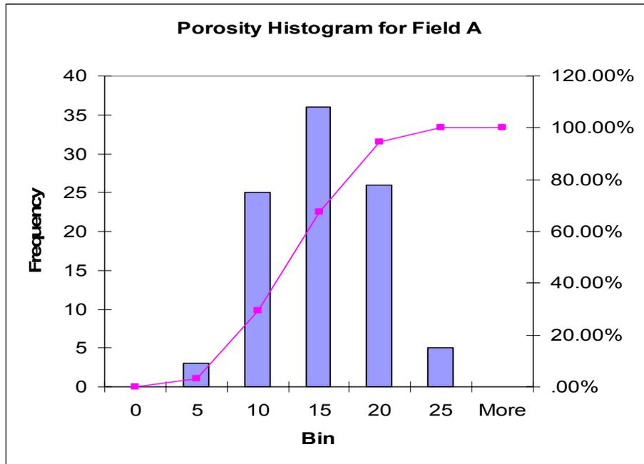
Figure B.2- Porosity Distribution Histogram for Field A
