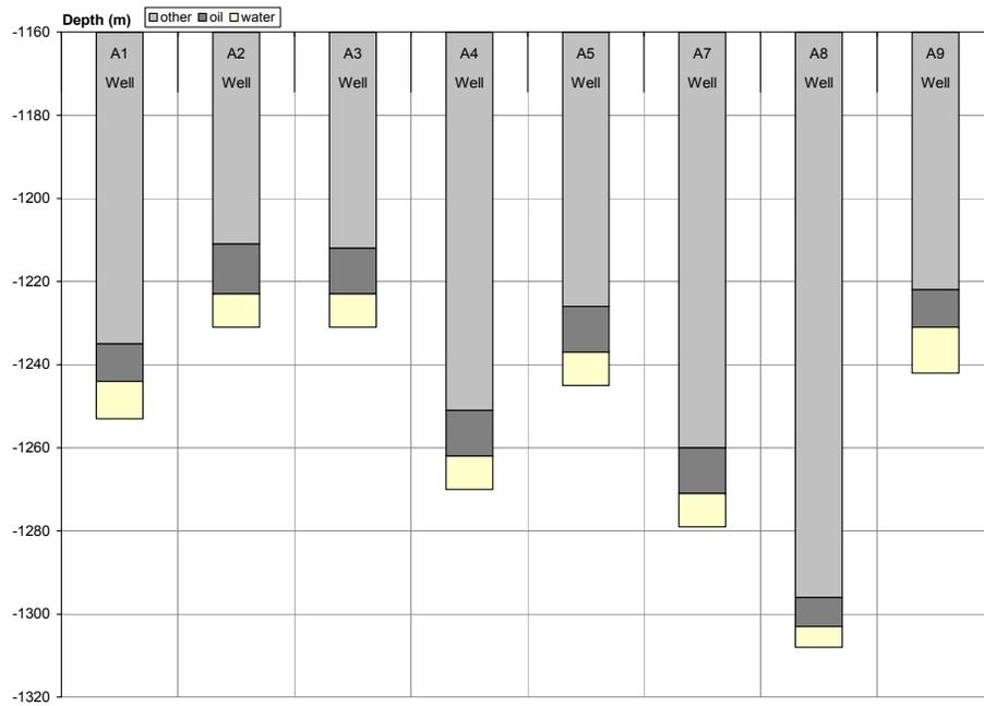
Figure B.1- Log Analysis Depth Plot for Field A
