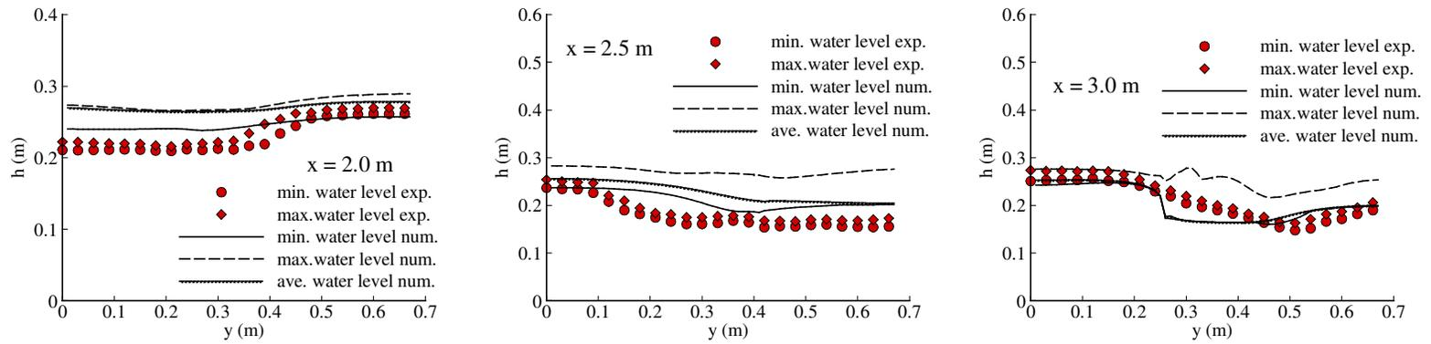
**Figure 4.18. Comparison of measured and computed water surface profiles at certain cross-sections, Case C1**
