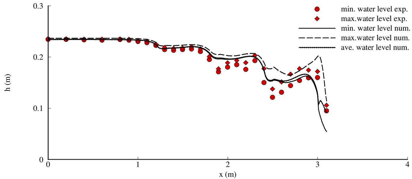
**Figure 4.15. Comparison of measured and computed water surface profiles along the channel centerline, Case B1**
