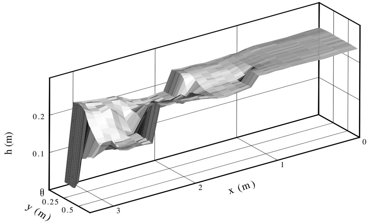
**Figure 2.7. Water surface profile of experimental case B1**
