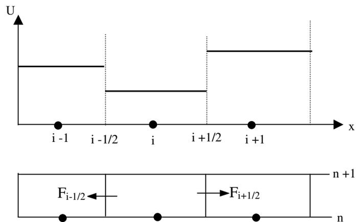
**Figure 3.2. Upwind method for one-dimensional flow**
