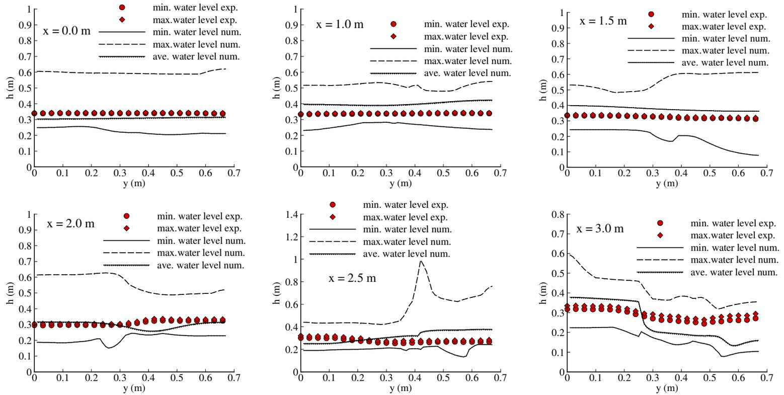
**Figure 4.20.** Comparison of measured and computed water surface profiles at certain cross-sections, Case C2
