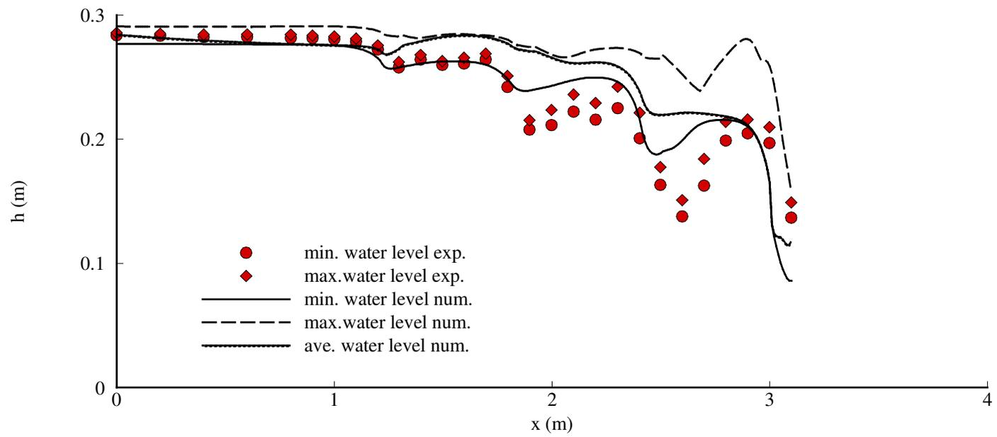
**Figure 4.19. Comparison of measured and computed water surface profiles along the channel centerline, Case C1**
