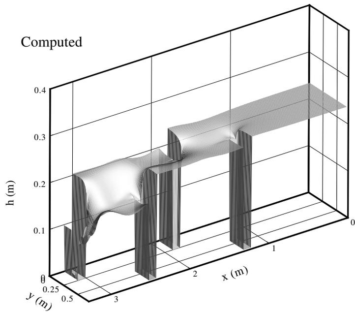
**Figure 4.6. Water surface profiles, Case B1**
