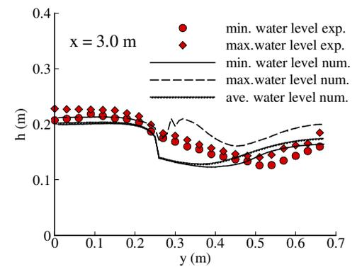
**Figure 4.14. Comparison of measured and computed water surface profiles at certain cross-sections, Case B1**
