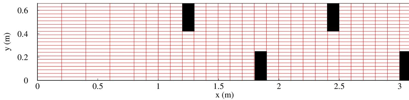
**Figure 2.4. Plan view of the measuring channel with measuring points indicated by intersections of the gridlines**
