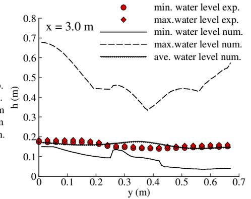
Figure 4.12. Comparison of measured and computed water surface profiles at certain cross-sections, Case A2
