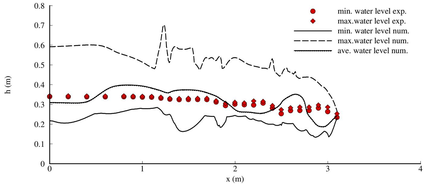
**Figure 4.21. Comparison of measured and computed water surface profiles along the channel centerline, Case C2**
