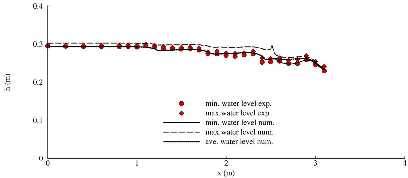
**Figure 4.17. Comparison of measured and computed water surface profiles along the channel centerline, Case B2**
