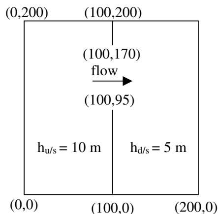
**Figure 4.2. Definition of problem domain for two-dimensional dam break, Test Case 3.**
