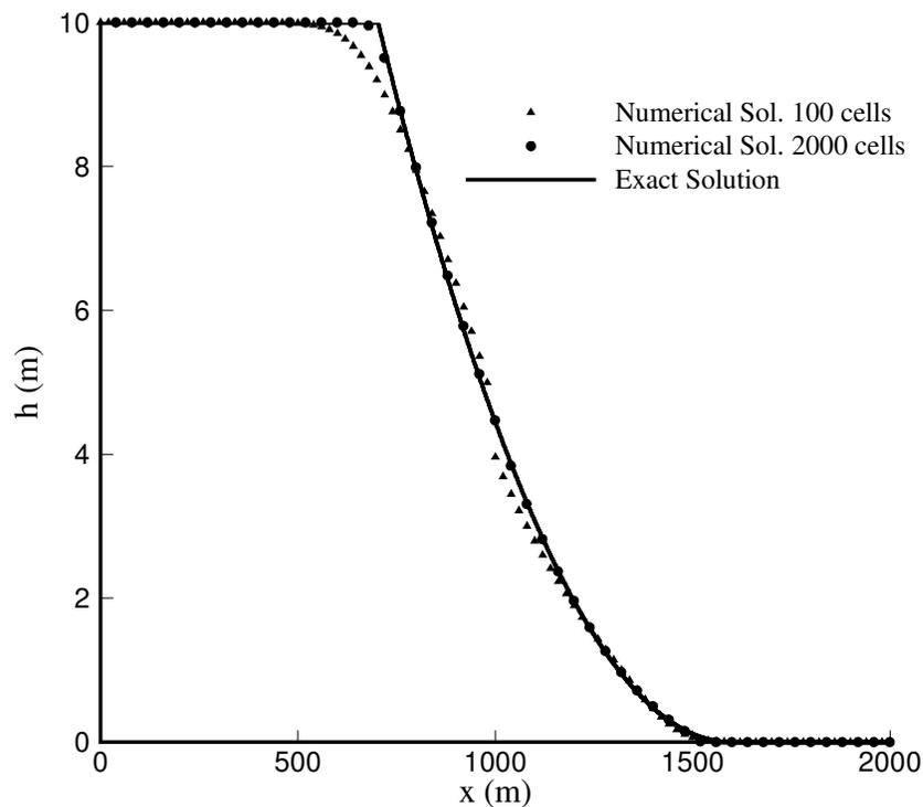
**Figure 4.1. Comparison of analytical and numerical solutions of one-dimensional dam break problem, Test Case 2.**
