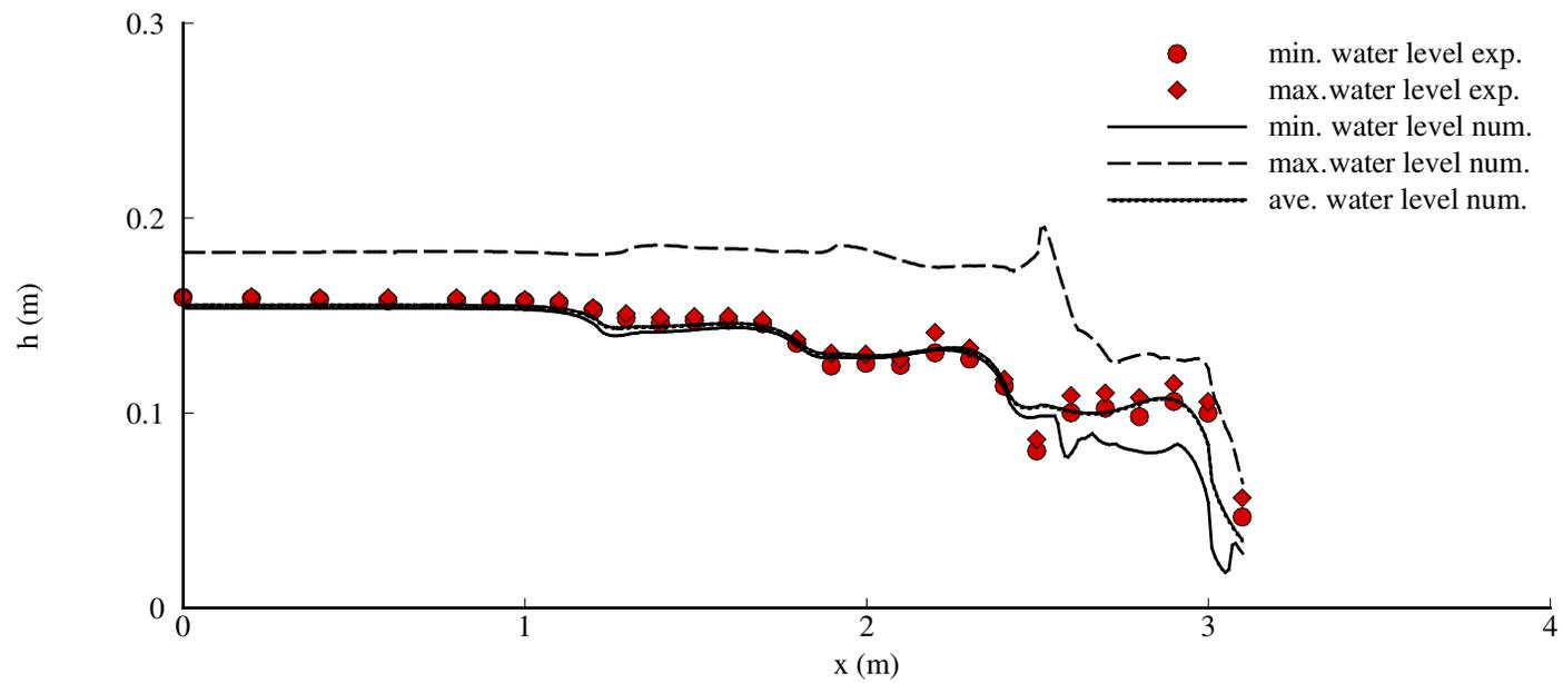
**Figure 4.11. Comparison of measured and computed water surface profiles along the channel centerline, Case A1**
