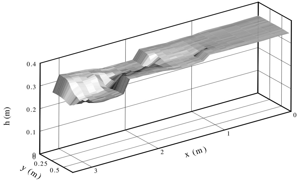
**Figure 2.10. Water surface profile of experimental case C2**
