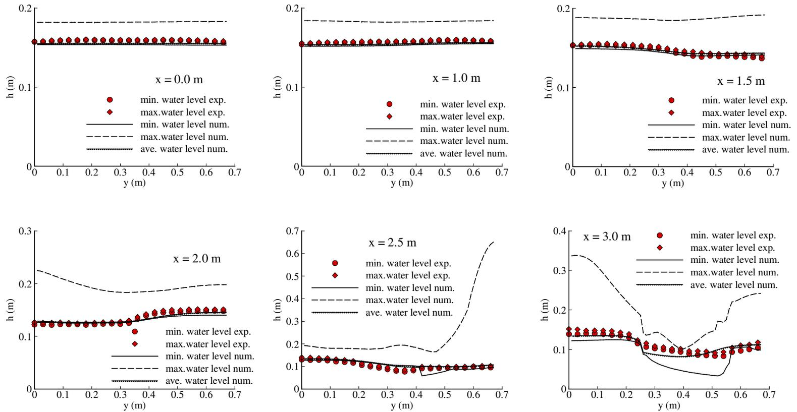
**Figure 4.10.** Comparison of measured and computed water surface profiles at certain cross-sections, Case A1
