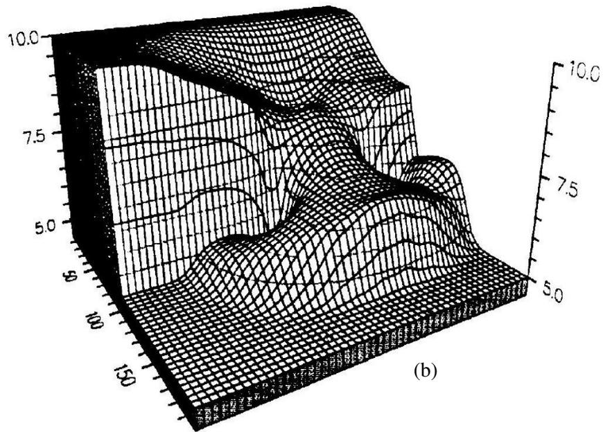
**Figure 4.3. Surface plot of two-dimensional dam break problem, Test Case 3 (a) Solution with the current model. (b) Solution by Anastasiou and Chan (1997).**
