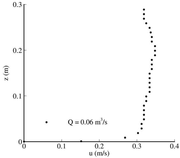
Figure 2.2. Vertical velocity distribution at the midpoint of inlet section
