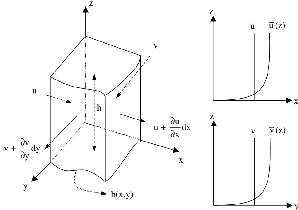
**Figure 3.1. Flow with a free surface under gravity**
