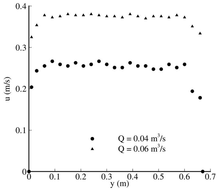
Figure 2.3. Velocity profile at the inlet section across the cross-section
