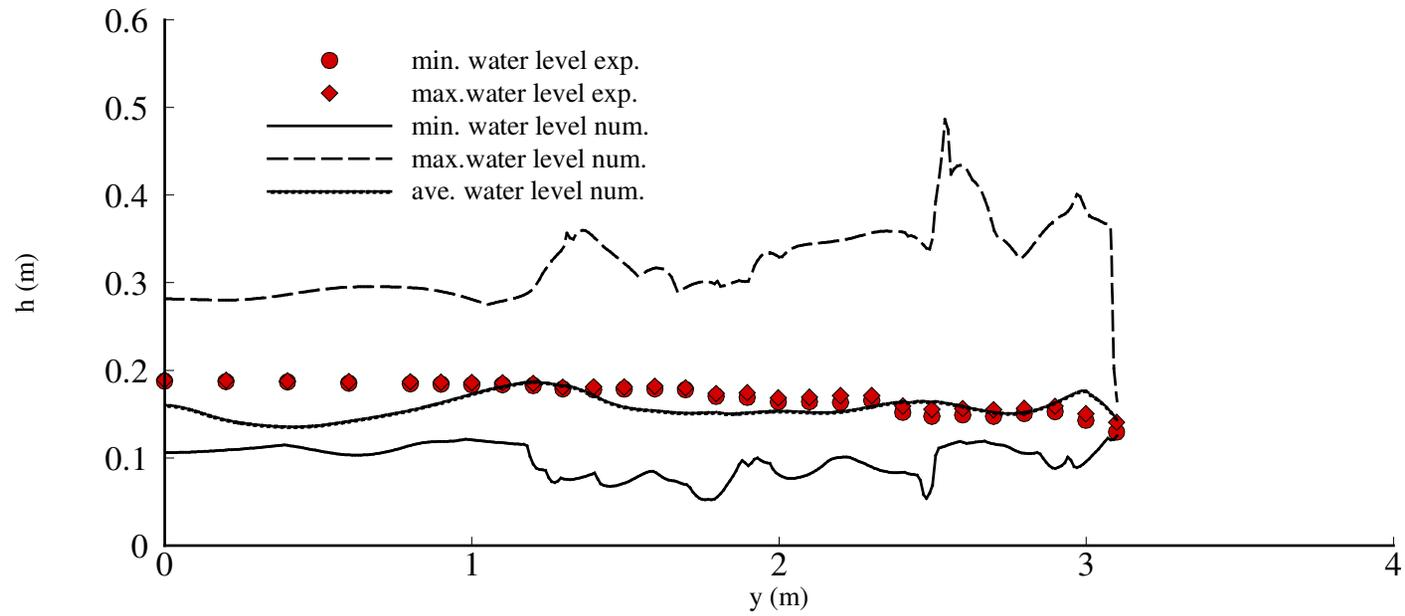
Figure 4.13. Comparison of measured and computed water surface profiles along the channel centerline, Case A2
