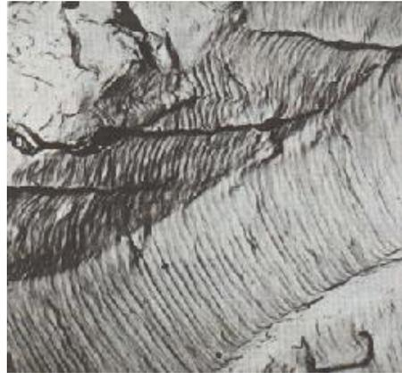
Figure 2.10 Example of the Striations Found in Fatigue Fracture [4]
