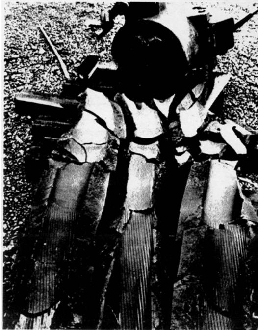
Figure 1.1 Fractured Gun Tube [1]
