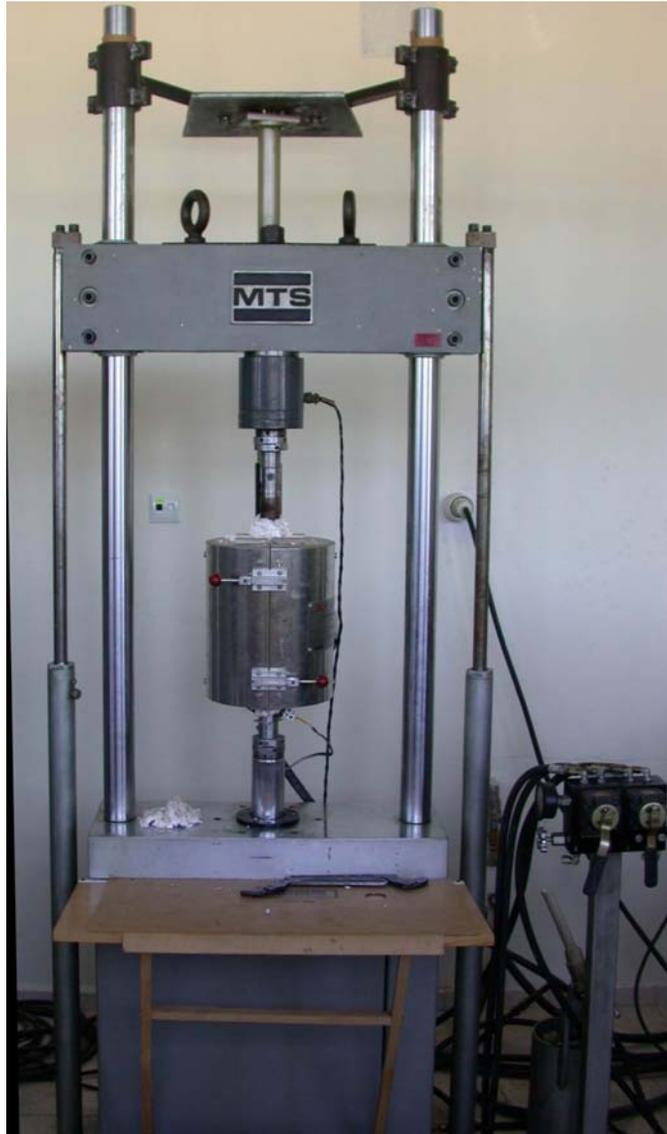
Figure 3.5 Furnace Attached to MTS Testing Machine
