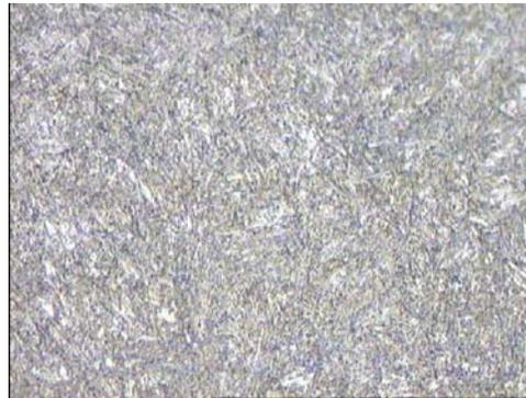
Figure 4.9 Microstructure of Specimen After Fatigue Test at 400<sup>0</sup>C and 0.2% Strain Amplitude (50X)
