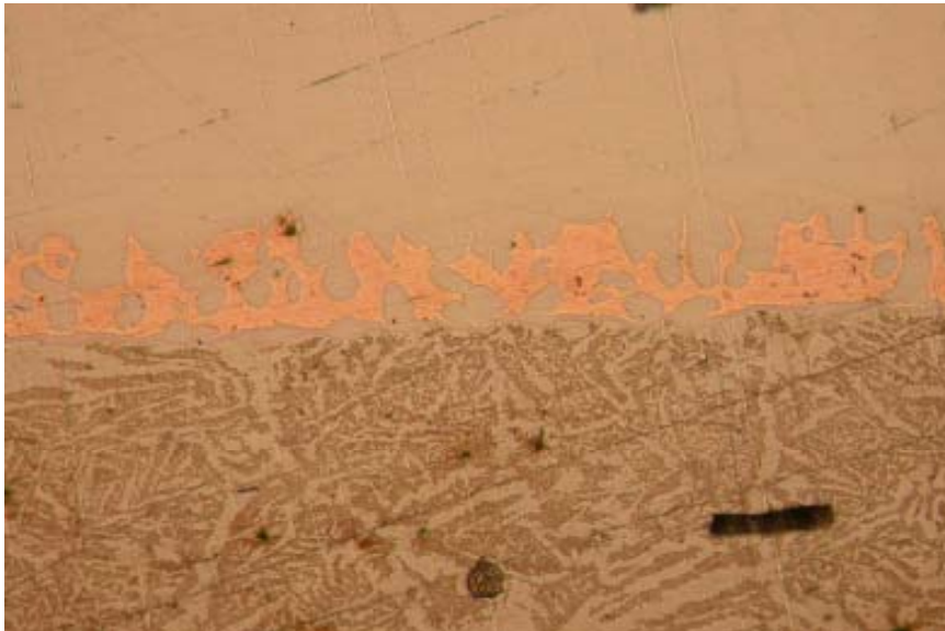
Fig. 7.5 x200 Optical Microscope Image of Cu-24 wt % Ni Brazed Region
