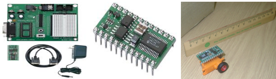
Figure 3.1 Basic Stamp II kit, BS2-IC and first prototype of MinT-DB [85].
