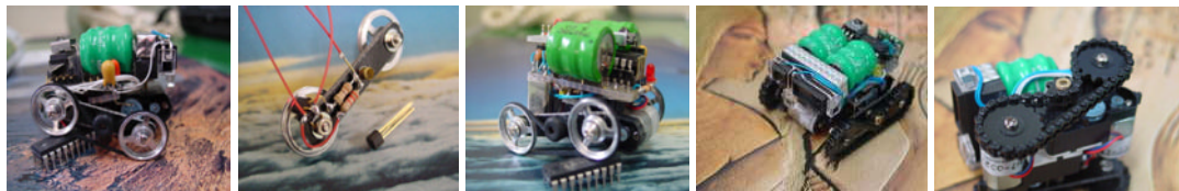
Figure 2.9 Wheels with encoders and unique suspension system development [37].
