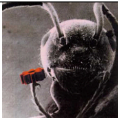
Figure 1.1 Ant and gear produced by LIGA Technology of MEMS [3].
