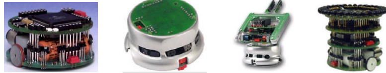
Figure 2.14 Khepera robots and modularity [44 and 45].
