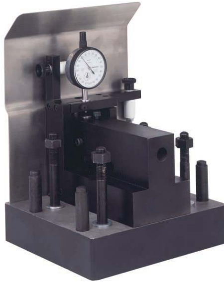
Figure 3.4: Lathe tool dynamometer setup.
