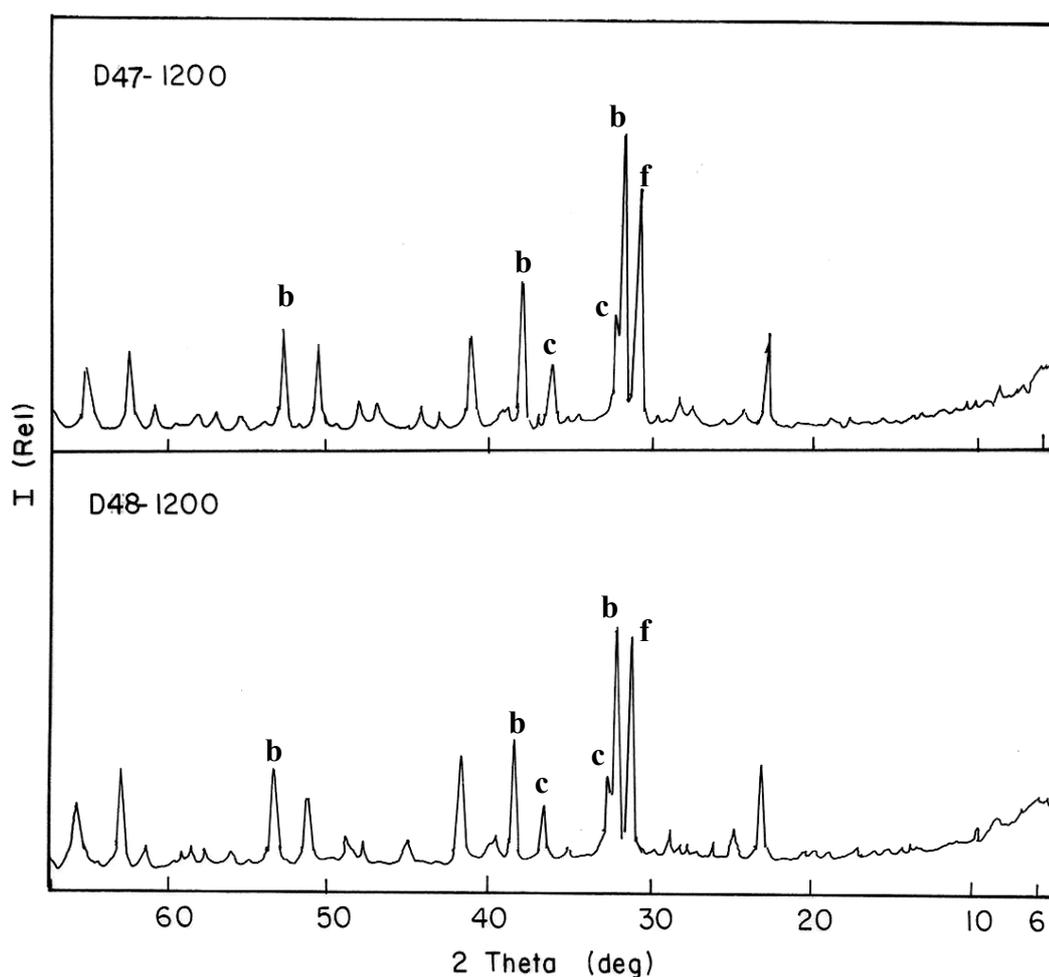
Figure 3.6 The X-ray Powder Diffraction Pattern of the Products Obtained From the Flux Reactions at 1200 °C (**Exp.No:D47, D48**), respectively (where b=Sr<sub>7</sub>Zr(PO<sub>4</sub>)<sub>6</sub>, c=ZrO<sub>2</sub>, f= Sr<sub>3</sub>(PO<sub>4</sub>)<sub>2</sub>)
