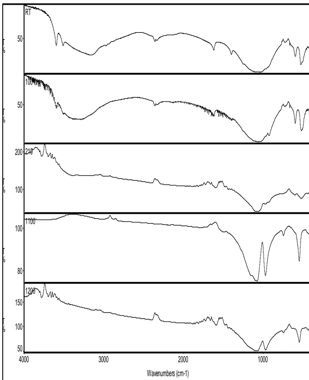
Figure 3.11 The IR Spectra of the Products Obtained From the Reactions of  $ZrO_2 + SrCO_3 + H_3BO_3 + (NH_4)_2HPO_4$  After Filtering at Room Temperature, 100 °C, 210 °C, 1100 °C, 1200 °C, respectively
