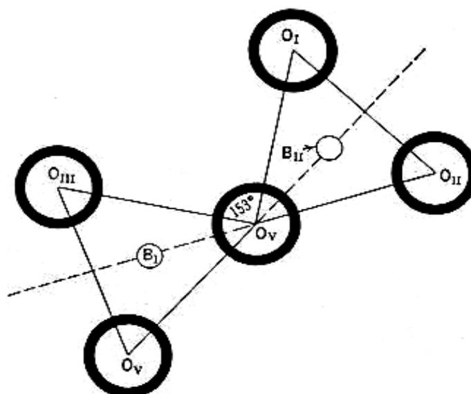
Figure 1.2 The Crystal Structure of Pyroborate [8,9]
