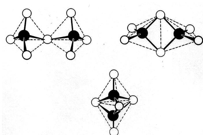
Figure 1.4 Condensed  $\text{PO}_4$  Tetrahedra. **a)** Corner Sharing, **b)** Edge Sharing, **c)** Face Sharing [24]
