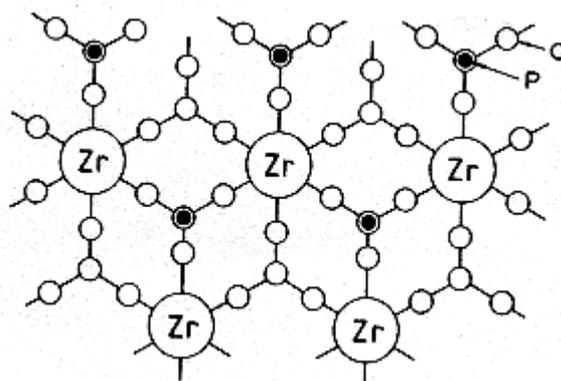
Figure 3.13 Structure of Zirconium Phosphate [42]
