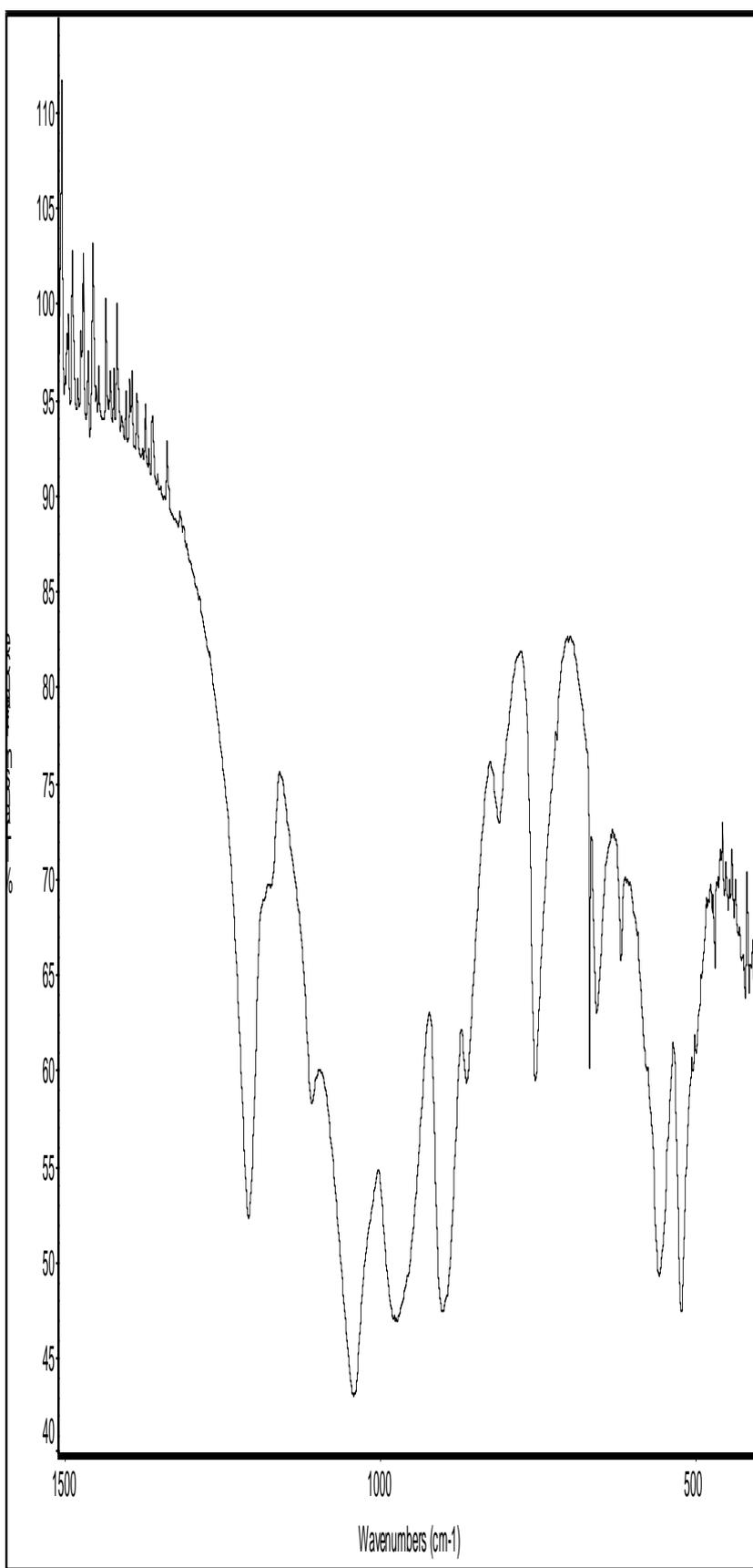
Figure 3.3 The IR Spectra of the Products Obtained From the Solid State Reactions of  $2\text{ZrO}_2 + 2\text{SrCO}_3 + \text{B}_2\text{O}_3 + 4)_2\text{HPO}_4$  at  $950^\circ\text{C}$
