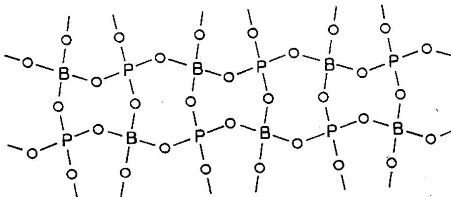
Figure 1.5 Boron Phosphate, Projected on to a Plane [42]
