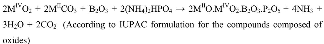
In the case of  $M^{IV}=Zr^{4+}$  and  $M^{II}=Sr^{2+}$ , the formation of  $ZrSr[BPO_7]$  was observed together with  $ZrO_2$  and  $SrBPO_5$ . The formation of a new phase was proved
