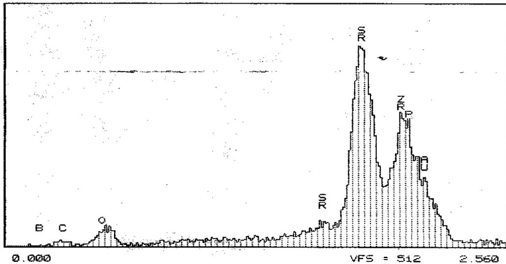
Figure 3.2 EDX Spectrum of the Products Obtained From the Reaction of  $2\text{ZrO}_2 + 2\text{SrCO}_3 + \text{B}_2\text{O}_3$  with  $2(\text{NH}_4)_2\text{HPO}_4$  at  $950^\circ\text{C}$
