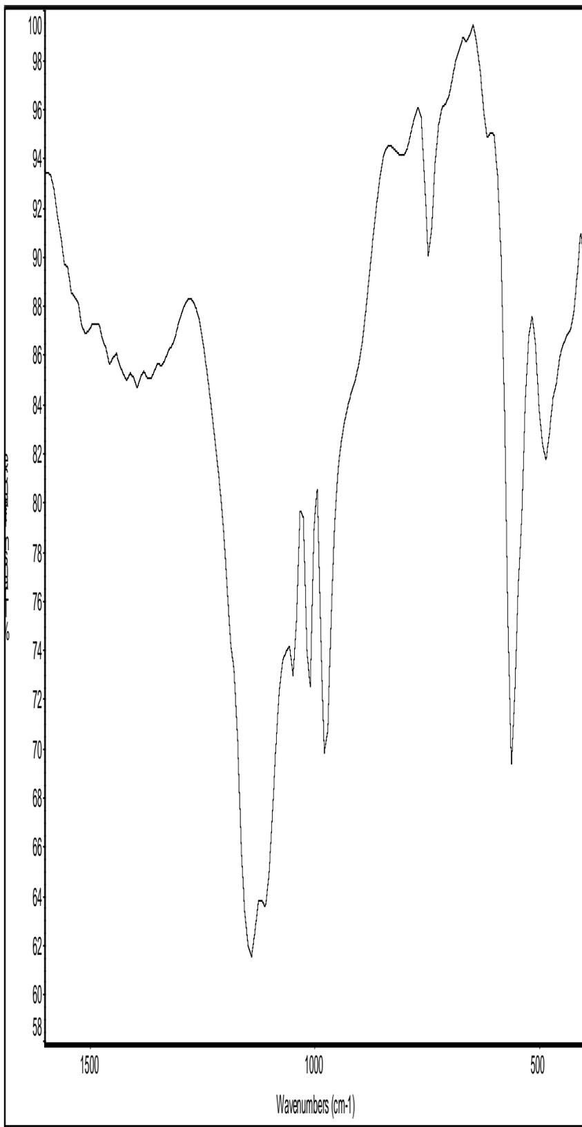
Figure 3.10 The IR Spectrum of the Products Obtained From the Solid State Reactions of  $2\text{SiO}_2 + 2\text{SrCO}_3 + \text{B}_2\text{O}_3$  with  $2(\text{NH}_4)_2\text{HPO}_4$  at  $1100\text{ }^\circ\text{C}$
