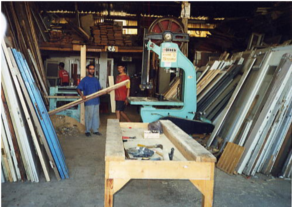
Figure 4.4 Workshop for repairing used timber fenestration and door sets (Izmir) (Elias-Özkan and Düzgüneş, 2002).
