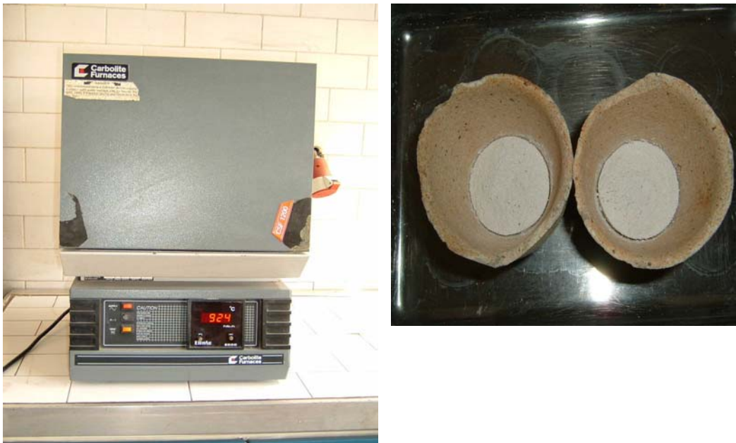
Figure 3.2. The muffle furnace and roasts in the crucible
