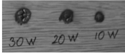
Figure 6.14- Burn patterns of laser beam on wood for 10W, 20 W and 30 W
